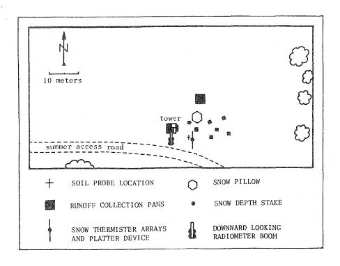
Figure 1. Schematic diagram of the Mammoth Mt. instrument site.
