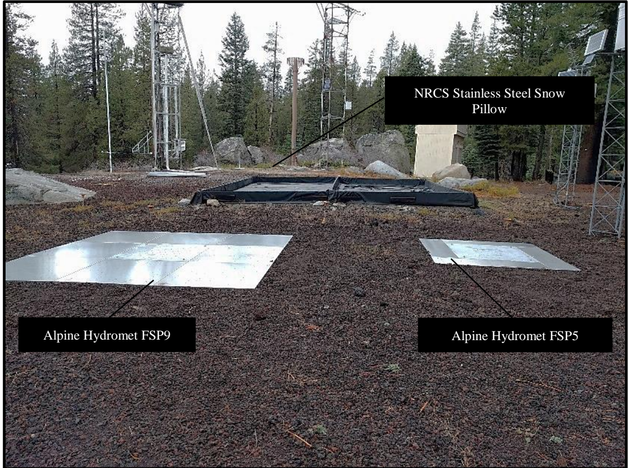
Figure 1. 2018 UCB Central Sierra Snow Lab 2016-17 sensor configuration
