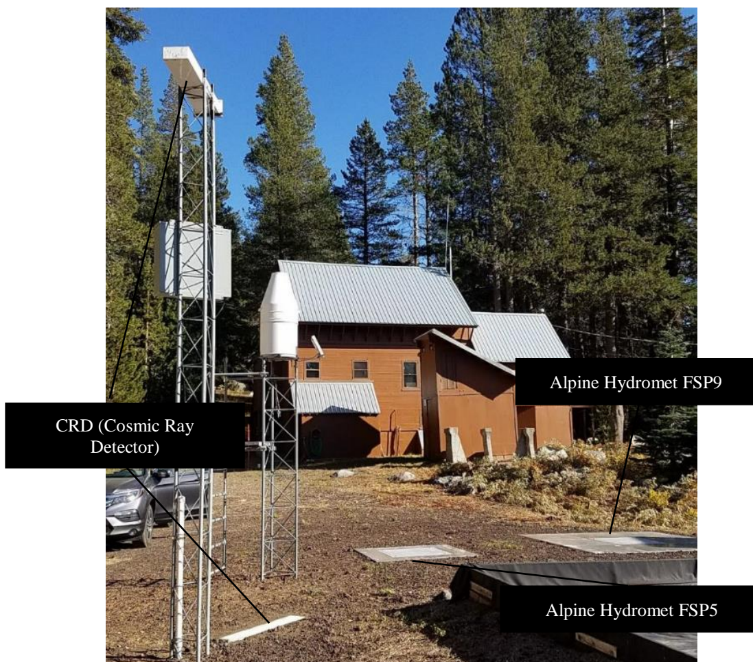
Figure 2. UCB Central Sierra Snow Lab 2017-18 with the addition of the CRD ground and reference detector
