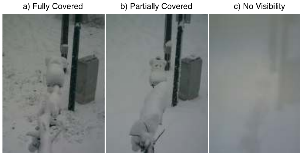
Figure 1. Time lapse photos of the ventilated 4-stream radiometer at Snoqualmie Pass demonstrating different SOD classification used in the algorithm evaluation.
