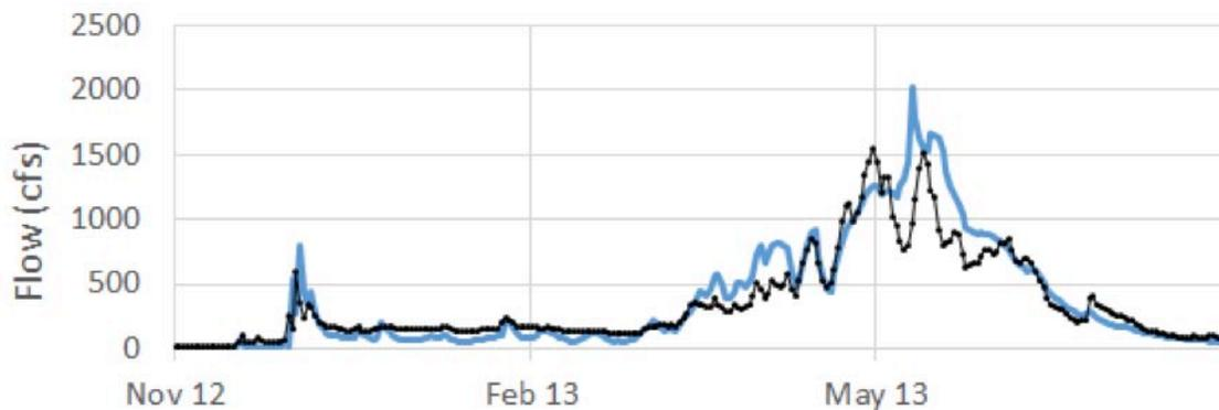
Figure 2. Modeled and observed streamflow on Tuolumne River above California's Hetch Hetchy Reservoir, using ParBal plus North American Land Data Assimilation System (Xia et al., 2012) precipitation as input. Modeled values are in blue, observed in black.
