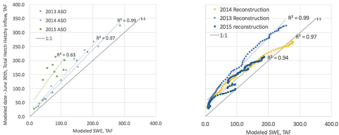
Figure 1. Modeled SWE vs. unimpaired total inflow into Hetch Hetchy Reservoir from ASO and reconstruction. Comparisons with ASO data are in the left figure, comparisons with reconstruction in the right.
