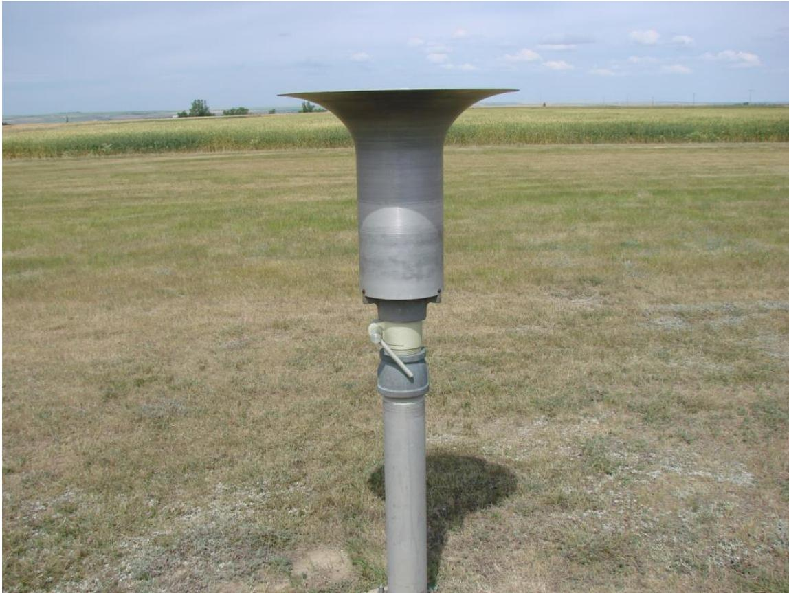
Figure 3. A Nipher-shielded precipitation gauge at the Swift Current Agricultural Research Centre farm.
