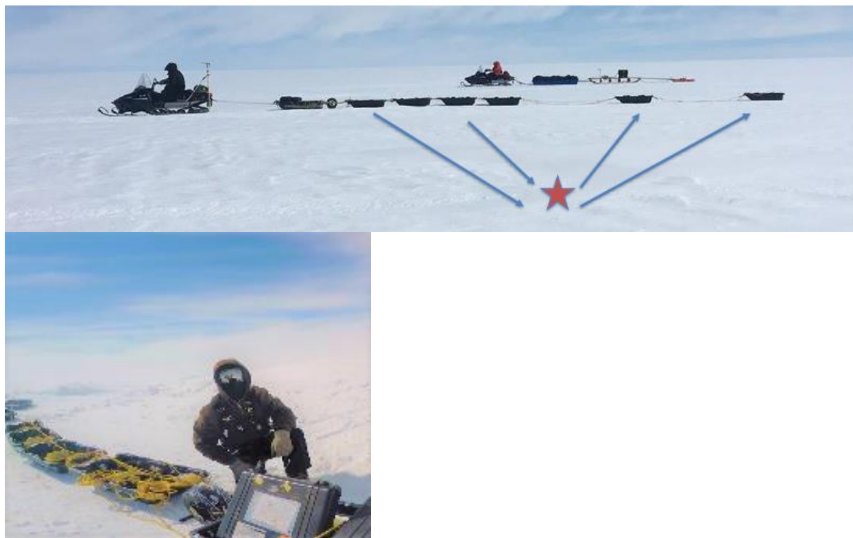
Figure 1. The multi-offset radar in operation (top) and under repair (bottom) during the 2016 GreenTrACS campaign. The star (top) represents the CMP location
