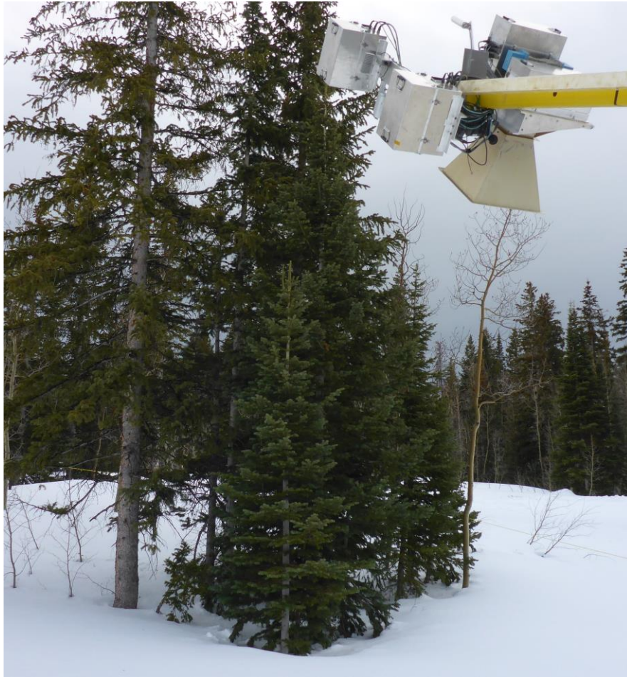
Figure 3. The evergreen trees brightness measurement by the microwave radiometer on Feb 10, 2017. The air temperature is above freezing, and there is no snow on the trees.
