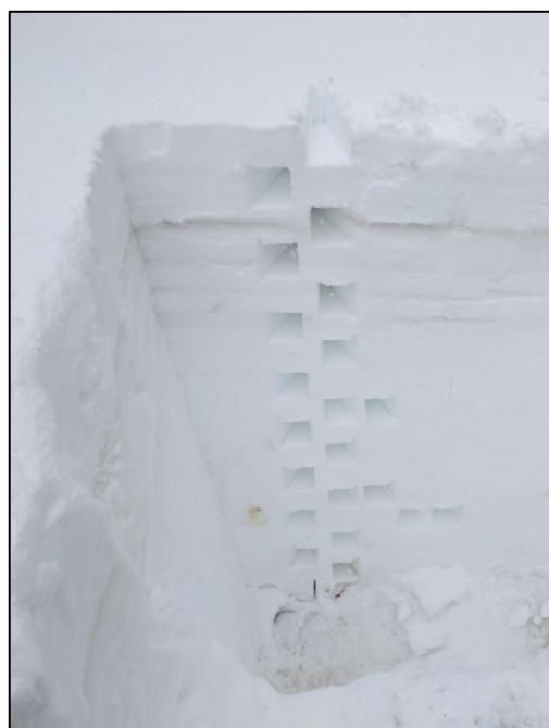
Figure 2. Picture of snow pit in upper Parleys showing 1-L density cuts for SWE and snow sampling. A combined dust layer (D1-3) can be seen as a distinct darker layer below ~20 cm of new snow.
