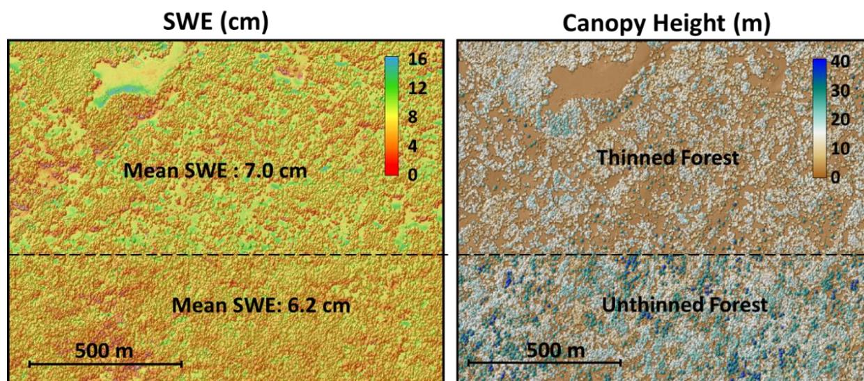
Figure 2. **Left:** SWE distribution across a managed forest boundary at a site with flat topography in the mid-elevation LiDAR box showing the average SWE in the thinned and unthinned parts of the image. **Right:** Canopy height for the area. Note the canopy hillshade effect on both maps to emphasize the locations of trees.
