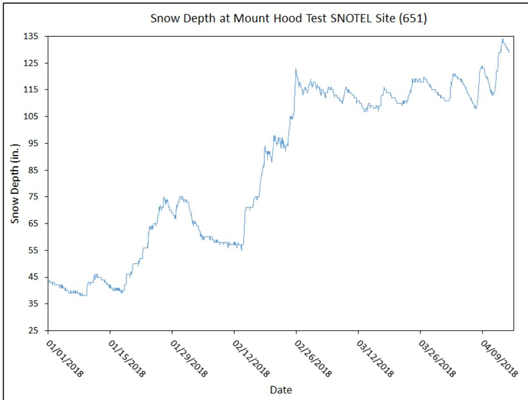
Figure 1. Example of the data collected by an in-situ ultrasonic snow depth sensor.
