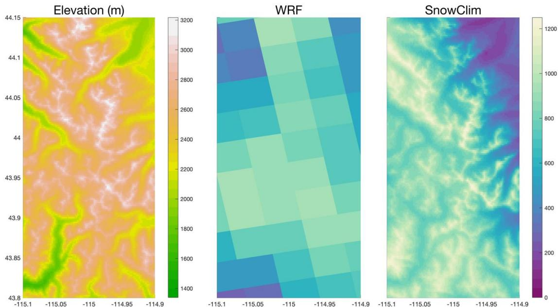
Figure 2. For an area of the Sawtooth Mountains in Central Idaho, a) terrain elevation (m), b) average historical SWE in the month of April as modeled by WRF at 4km resolution, and c) average historical April SWE (mm) as modeled by SnowClim at 210m/1050m resolution. The color scale is the same for b) and c).
