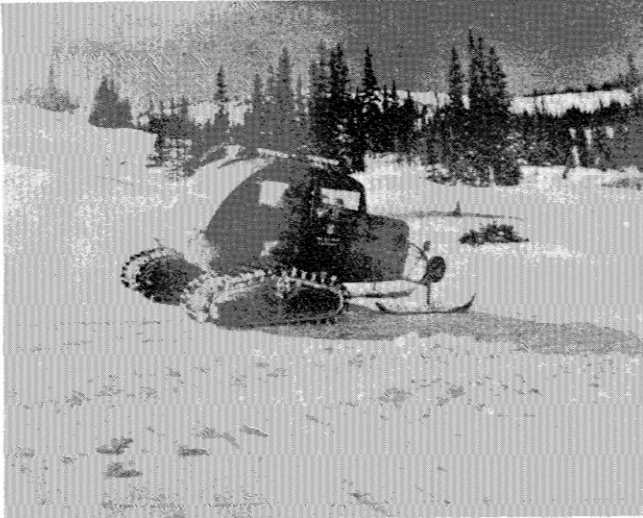
Figure 1.-- Two Pontoon Tucker Sno-Cat. This machine and earlier models have been used for several years in the west.
