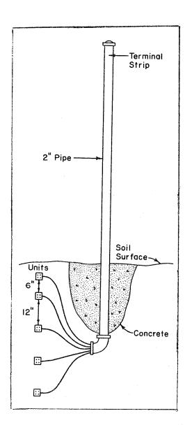
Figure 1. Sketch of a Typical Soil Moisture Station.
