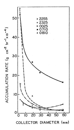
Figure 1--Rime accumulation rates on cylinders of different diameters, March 5, 1970.
