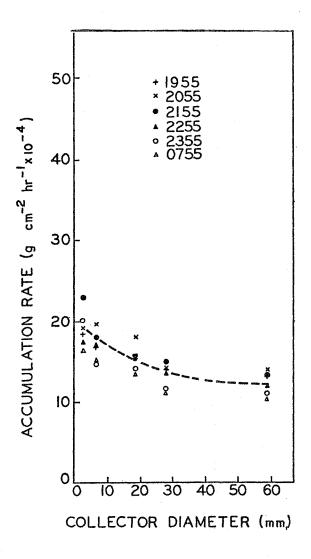
Figure 2--Hoarfrost accumulation rates on cylinders of different diameters, March 4, 1970.
