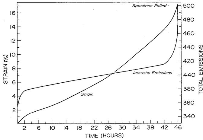
Figure 3. Strain and acoustic response of a snow sample subjected to a constant uniaxial tensile stress of 20.5 kilonewtons per square meter.
