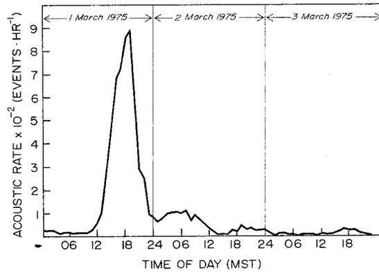
Figure 5. Acoustic rate response observed over a three-day period in early March 1975. This record is typical of the acoustic activity observed throughout our winter field testing program.
