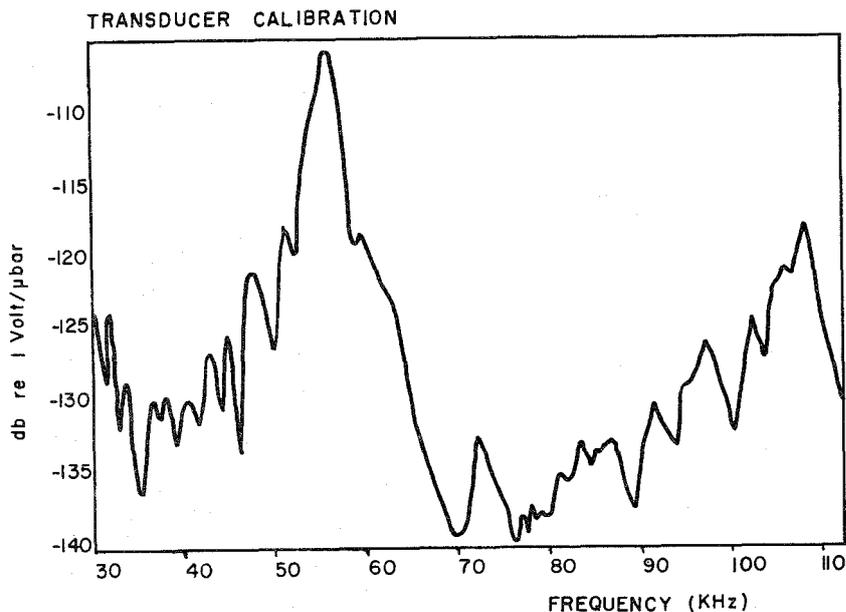
Figure 1. Response versus frequency curve for a typical acoustic emission transducer used to monitor acoustic emissions from snow.
