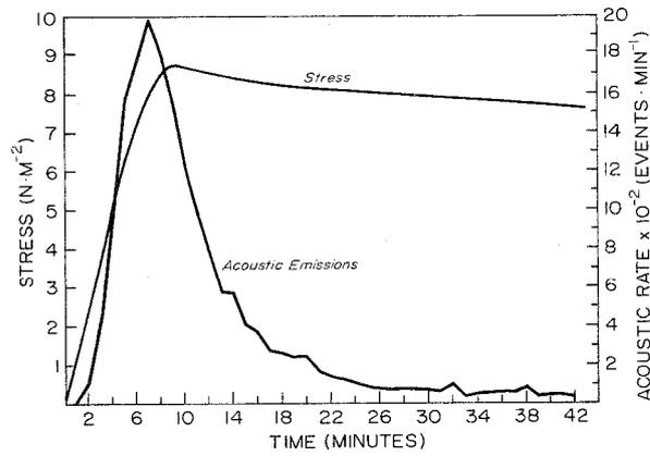
Figure 4. Stress and acoustic rate response for a snow sample deformed at a constant rate of  $1.54 \times 10^{-4}$  m.min<sup>-1</sup>.
