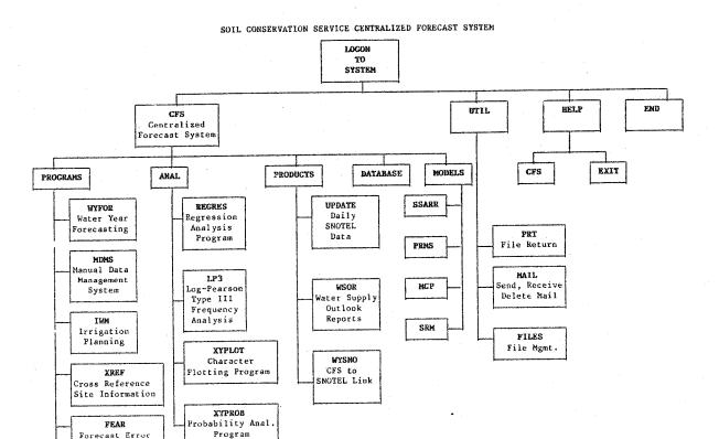
Figure 2. Block diagram of the CFS menu structure. Words in bold face are menu commands.
