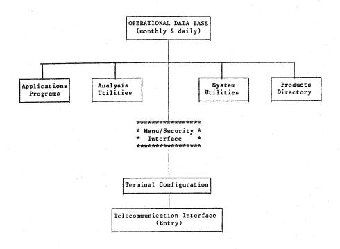
Figure 1. Block diagram of the major functional components comprising CFS as viewed by a dial-in user.
