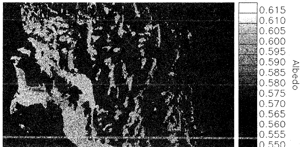
Figure 7 Snow albedo retrieved from algal concentration (Figure 5) using the model represented by equation (7). Snow-free areas have been masked from analysis.
