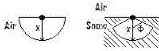
Figure 1: Difference in the shape of a radar pulse traveling through air (left) and passing from air to snow (right), where x is the traveled distance and \Phi is the largest angle of refraction.
