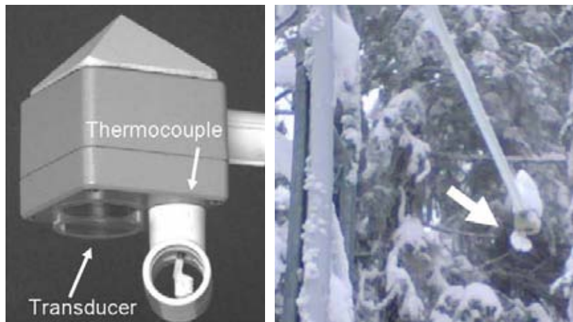
Figure 6. Judd USDS close-up (left), Quartz Peak SNOTEL depth sensor with snow build-up on thermocouple that obstructed the transducer (right).
