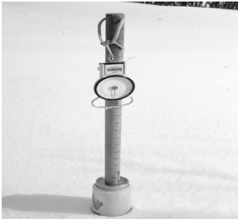
Figure 2. Dowel inserted into bottle for lower pressure measurements.
