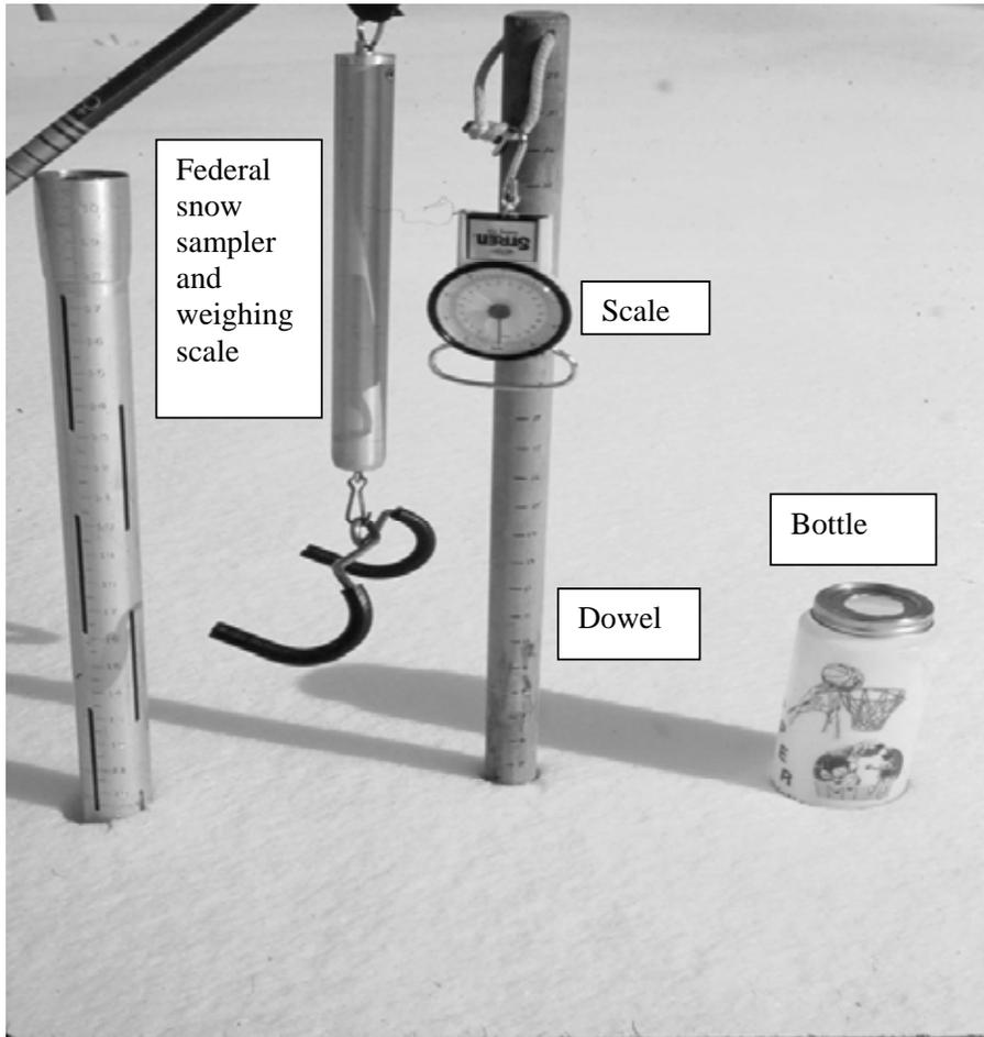
Figure 1. Equipment used for the snow sinking studies.
