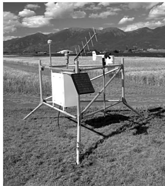
Figure 2. Typical AgriMet Weather Station
