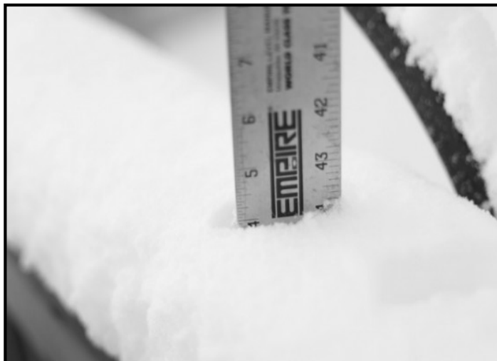
Figure 2. Measuring daily snowfall on a snow board with a ruler.
