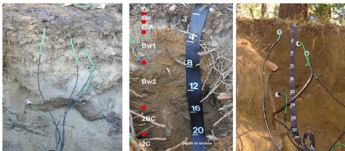
Figure 1. Soil Moisture sensor placement at NRCS SNOTEL sites.
